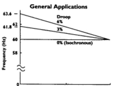
Many applications easily accept some speed droop which means a less costly and complex governor can be used, even if the gen set will be paralleled with other units.
